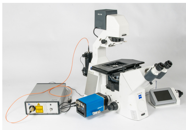
Figure 35: Microscope set-up example (Zeiss AxioObserver Z1, inverse widefield fluorescence microscope, courtesy of Zeiss AG) with Rapp OptoElectronic laser light source and combined de-speckling and optical coupling unit, with a pco.flim camera connected to the microscope and the laser light source.
