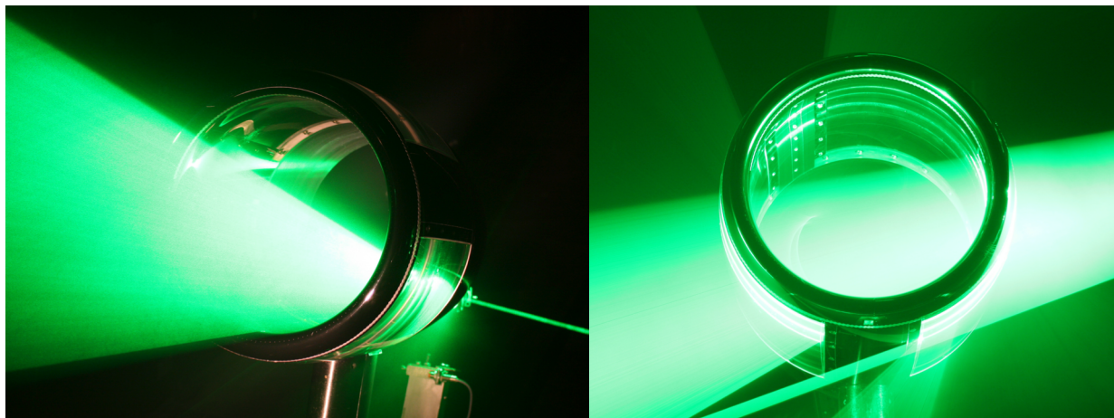
(a) Light sheet in main flow direction (b) Light sheet perpendicular to the x -axis Fig. 3 Complementary light sheets
