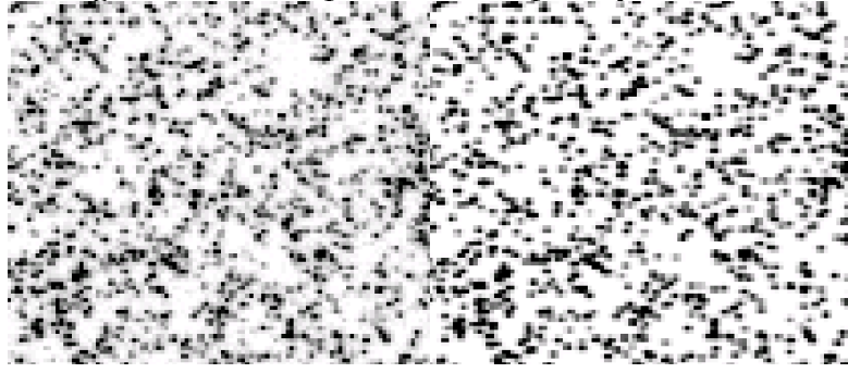
Figure 7: (Left) detail from camera image; (right) reprojection of particle distribution as reconstructed by STB.
