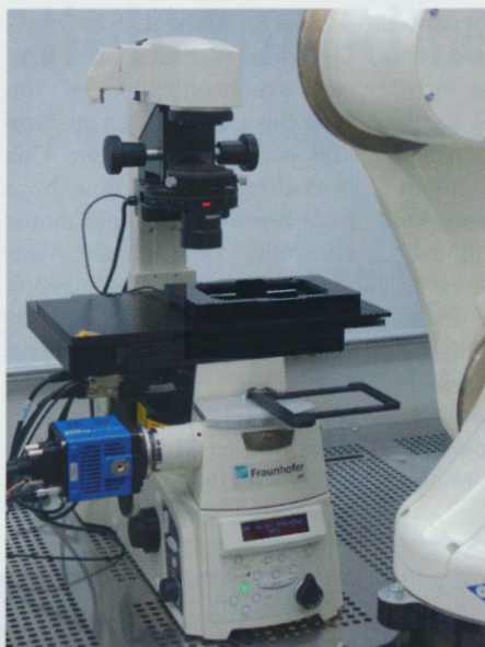
Fig. 1: High-speed microscope inside an automated production facility for iPS cells.
