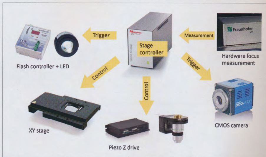
Fig.3: The basic design of the modular high-speed microscope (Image: Fraunhofer IPT).
