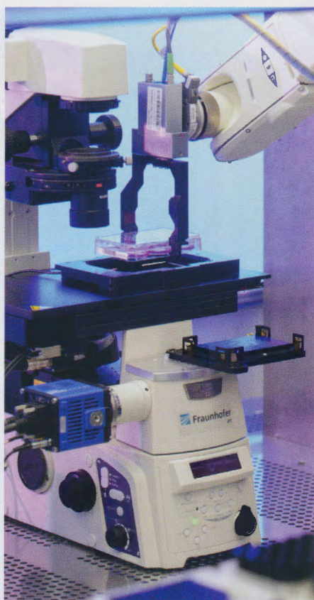
Fig.2: High-throughput microscopy systems: Large-surface objects can be microscopied within seconds. For the first time ever, 100-percent microscopic tests are now possible in the industrial environment. (Image: Fraunhofer IPT)
